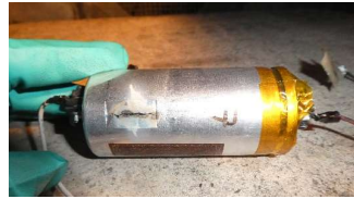
Cell after overcharge
