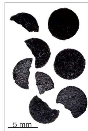
Delaminated and ruptured CCM + electrode powder
