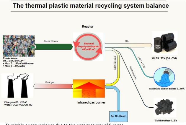
favorable energy balance due to the heat recovery of flue gas.
