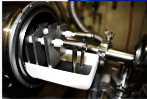
Tube furnaces with controlled atmosphere up to 1600°C for material testing
